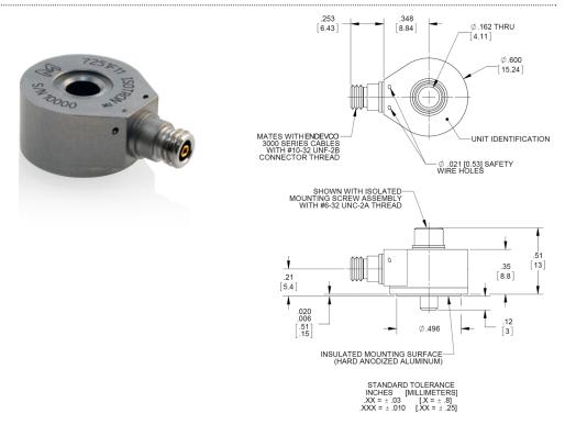
Model 7251FXX is a small piezoelectric accelerometer with integral electronics featuring IEEE P1451.4 Transducer Electronic Data Sheet (TEDS) capability. The unit is hermetically sealed against environmental contamination, offers high output sensitivity, and wide bandwidth. The centrally located mounting bolt permits 360° cable orientation, a very desirable feature in many applications. The lightweight design effectively minimizes mass loading effects on the test structure.
