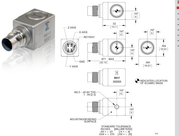
Endevco model 66N7 is a miniature triaxial piezoelectric accelerometer with integral hybrid electronics with transducer electronic data sheet (TEDS) capability. The accelerometer is packaged in a 10 by 10 by 13 mm case of welded titanium construction. One of the key design characteristics is the low unit-to-unit phase deviation at low frequency, ideal for modal analysis of large rigid bodies.
