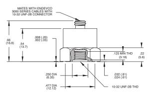
NOTE: IF ALTERNATE STUD IS USED, THE LENGTH OF STUD FROM MOUNTING SURFACE MUST BE .140/.135 (3.56/3.43)
