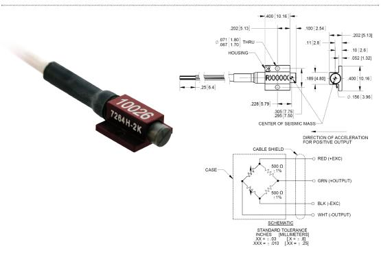
Model 7264H is a very low mass accelerometer weighing only 1.4 grams. This accelerometer is designed for crash testing and similar applications that require damping, broad frequency response, and minimum zero shift following the event. It is equivalent in form and fit to the Endevco model 7264C-2K in that the location of the center of seismic mass is the same.
