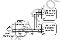
Serial Communication block diagram
