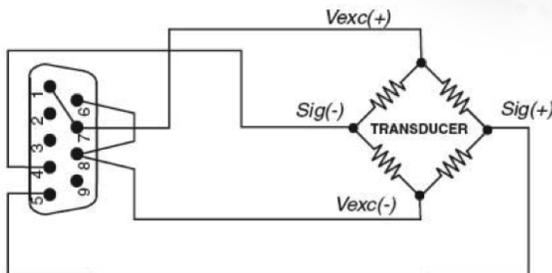
The model 126 is a microprocessor-controlled, 3-channel DC signal conditioner amplifier designed to be used with bridge type or differential output accelerometers and pressure transducers. The model 126 incorporates variable gain adjustment, shunt calibration capability, and multiple excitation level settings.
