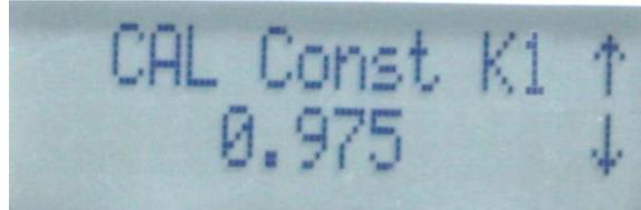
Figure 13: Calibration Constant screen
