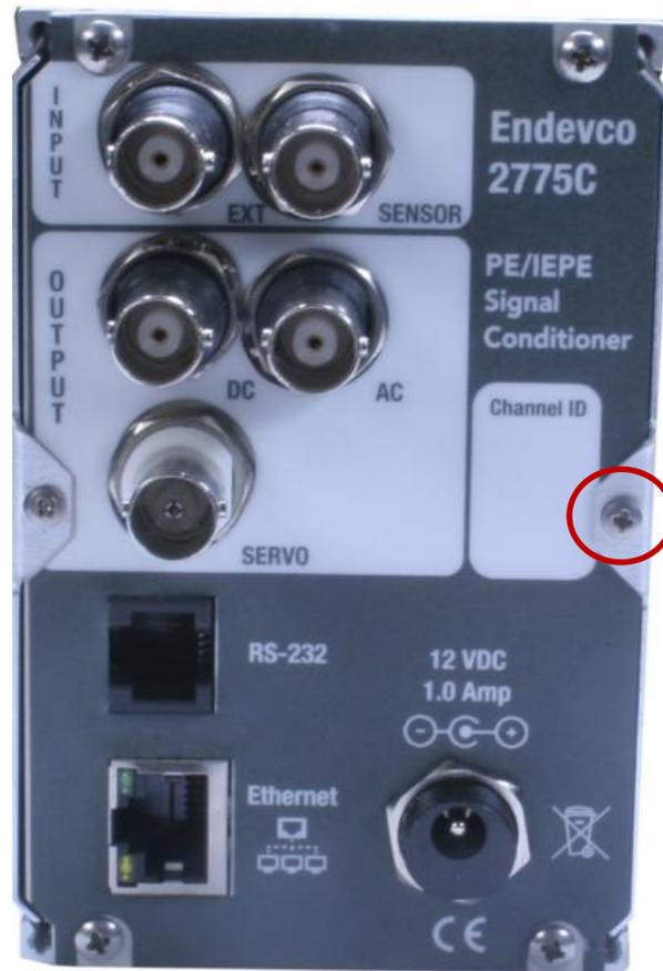
For internal switch access, remove this screw to allow side panel to slide back off unit
