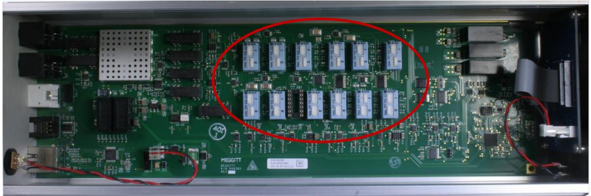
Figure 3: Filter and integrator switches
