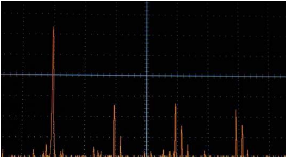
Figure 3C: FFT showing a distorted sine wave in the frequency domain
