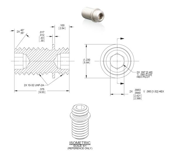
Mounting stud with hex socket head for use with accelerometers with a 10-32 thread.
