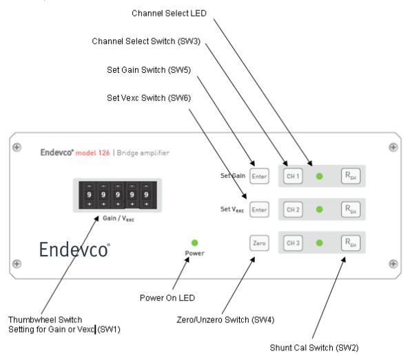
SW1 (gain / excitation) SW2 (shunt cal switch) SW3 (channel select switch) LED1 (channel select LED) SW4 (zero / unzero switch) SW5 (set gain switch) SW6 (set Vexc switch) LED2 (power on LED)
