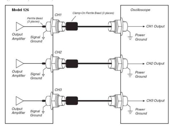
**Note**: The model 126 signal ground is isolated from power ground. This allows connecting the oscilloscope power ground to the 126 signal ground. To minimize high frequency EMI susceptibility, install clamp-on ferrites with frequency bands of 80 MHz to 800 MHz
