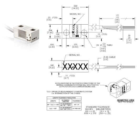
The ENDEVCO® Model 7274 series is a family of rugged, undamped, piezoresistive triaxial accelerometers designed for high-acceleration shock measurements in three mutually perpendicular axes. This family uses three sensors that are packaged in a mutually orthogonal arrangement in a two bolt-mount housing which shares the same footprint and bolt pattern as ENDEVCO® Model 7270A. The housing boasts a robust eight conductor cable that can repeatedly withstand the high-acceleration shock environment.
