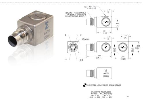
Endevco model 66FXX is a miniature triaxial piezoelectric accelerometer with integral hybrid electronics with transducer electronic data sheet (TEDS) capability. The accelerometer is packaged in a 10 by 10 by 13 mm case of welded titanium construction. One of the key design characteristics is the low unit-to-unit phase deviation at low frequency, ideal for modal analysis of large rigid bodies.
