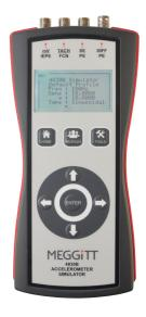
The 4830B accelerometer simulator is a hand held battery operated signal generator designed specifically to simulate the electrical output of common types of accelerometers. The instrument contains a highly accurate oscillator with an adjustable output level and is ideal for setting up, testing and the diagnosis of faults within data acquisition systems, FFT analyzers, environmental test systems or simply as a flexible signal generator.
