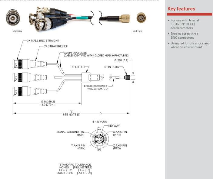
The convenient 3027AM3 breakout cable assembly provides accelerometer to measurement instrument interconnection. The accelerometer end of the assembly is made up of a lightweight 4-conductor shielded cable and a ¼-28, 4-pin plug to reduce mass loading. The instrumentation end consists of three rugged cables terminated with three BNC straight male plugs. Each plug is color-coded to identify the respective measurement axes.
