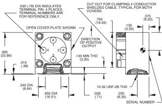
STANDARD TOLERANCE INCHES (MILLIMETERS) .XX = +/- .03 (.X = +/- .8) .XXX = +/- .010 (.XX = +/- .25)
