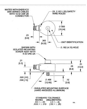
Model 7221A is a small, piezoelectric accelerometer designed specifically for general vibration measurement. The accelerometer offers wide bandwidth and operational temperature range, it is also hermetically sealed for high reliability. Its light weight (10.5 gm) effectively minimizes mass loading effects on small structures. This accelerometer is a self-generating device that requires no external power source for operation.
